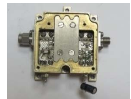
Figure 14 Fabricated RF PCBs
